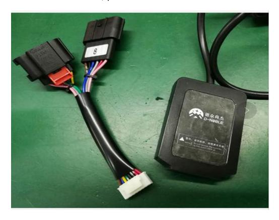
Pull out the Original car Gateway cable which will connect for Smart Module from Gateway connector . (Gateway cable is beside the accelerator)
