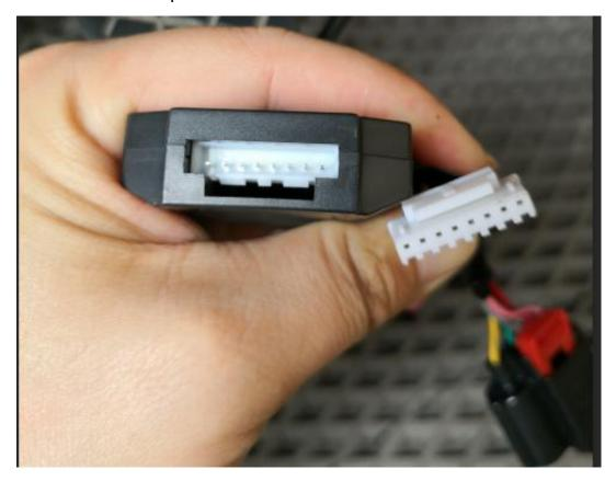
4. Connect the Smart Module cable to VW DVD's connector .
